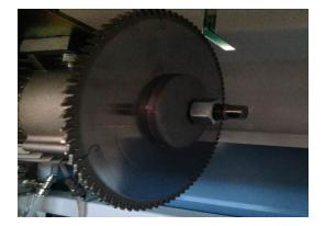
The stop system of the profile to be cut operates before that the blade moves so that to cover completely the exposed cutting part and to lock the piece to be cut. Control system with safety pedals. All control circuits which are in contact with the operator are in security low voltage 24 Vac. Safety protections against access to the dangerous parts of the machine according to the European norms.
