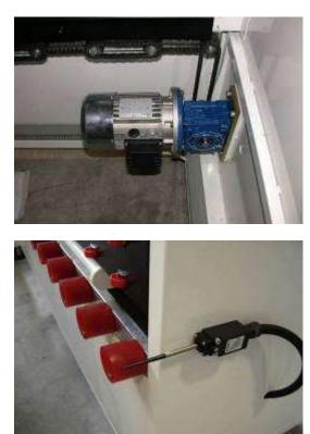
01 Washing machine with a length of 2 mt and height of 2 mt. Composed by 4 brushes diameter of 120 mm. with steel shafts, complete with two tanks with pumps, filters and internal in stainless steel. Heating water to 1.5 kW. Blower included in an insulated boxafono. Speed 4 mt per min.. The washer is open on the top. System of protection against access to dangerous parts of the machine according to European standards
