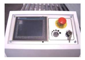
**EASY TOUCH SYSTEM** control panel that allows the operator to control the working process, to regulate the times and control the single operation of each component. Control circuits which are in contact with the operator are in security low voltage with bright panel on board machine. Protection against access to the dangerous parts of the machine according to EU norms.
