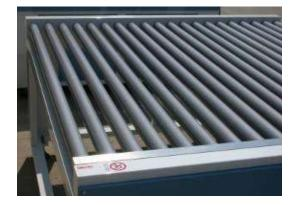
01 Pre-washing zone with a length of 1 mt. and height of 0,90 mt., with clutched anticut rollers, mounted on bearings and bushing in special plastic material, and stainless steel interior, complete the pre-wash with water to lose.
