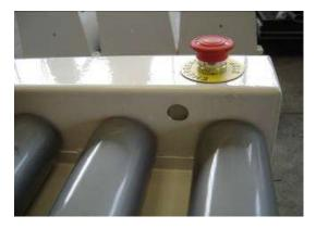
01 Motorized exit with a length of 2 mt. and height of 0,90 mt., with clutched anticut vulcollan rollers, mounted on bearings and bushing in special plastic material. This module has a motor complete of reducer. The four blowers are fed by two high pressure fans , stop glass system through sensor. Protections against access to the dangerous parts of the machine according to the EU norms.
