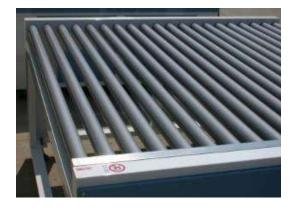
01 Pre-washing zone with a length of 1 mt. and height of 0,90 mt., with clutched anticut rollers, mounted on bearings and bushing in special plastic material, and stainless steel interior, complete the pre-wash with water to lose.
