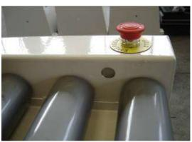
Motorized exit with a length of 2 mt. and height of 0,90 mt., with clutched anticut vulcollan rollers, mounted on bearings and bushing in special plastic material. This module has a motor complete of reducer. The four blowers are fed by two high pressure fans, stop glass system through sensor. Protections against access to the dangerous parts of the machine according to the EU norms.
