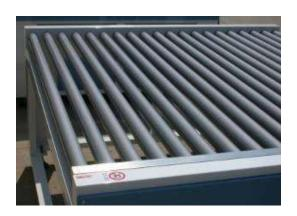
O1 Pre-washing zone with a length of 1 mt. and height of 0,90 mt., with clutched anticut rollers, mounted on bearings and bushing in special plastic material, and stainless steel interior, complete the pre-wash with water to lose.
